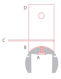
**4.** Connect one pole of the power supply to the power connector (C).
