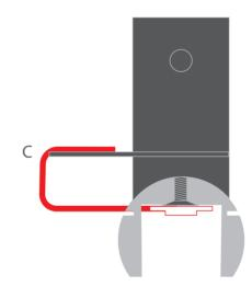
**5.** Insert the rod into the mounting bracket of the head. Block the rod by tightening the pressure screw in the head with the Allen wrench.
